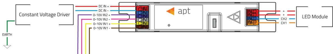
Figure 2 - APT-CV2-VD-LN Dual 0-10V Dimmer Configuration
