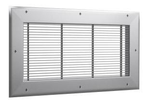
The SSLBG Series Linear Light Duty Bar Grille is designed for supply or return air in sidewall or sill installations. Designed with fixed 0° air foil blades parallel to the grille's long dimension, blades are reinforced on approximate 8" centers. Air foil blades are set at 0° on 3/8" centers allowing 1/4" spacing between blades.
