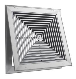
SSHFG CLCD Concentric Louvered Hinged Filter Grille is hinged in our 1000 Plaster Frame and secured with low profile 1/4-turn fasteners. The hinged filter grille allows easy access to filters or mechanical equipment. It is a high capacity, modular louvered face directional diffuser, which is highly configurable with multiple airflow patterns and optional features to tailor this product to specific applications.
